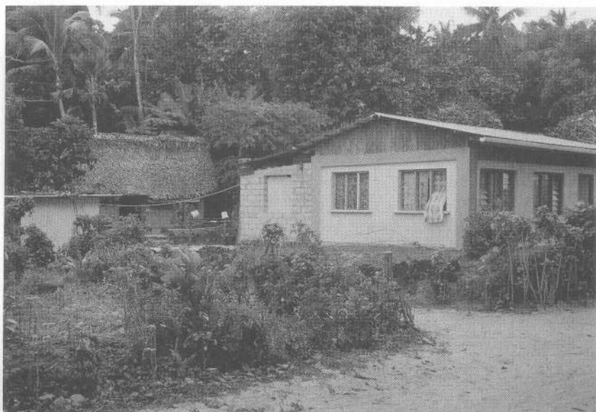
2.4 Contemporary Rotuman dwelling of cement, wood, and corrugated iron with louvered glass windows, showing new cement-block addition at rear. The house is on an elevated foundation surrounded by rocks; a border of croton plants decorates the front. Note also the thatched kitchen in the back, and the iron wash house. Jan Rensel, 1990.
